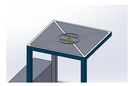
**Ammunition depot**: Prepared by each team, these shall be placed in an appointed location in the team's area and use specially designed tubes to supply 17mm bullets every 30-seconds to the team's robots. The end of the tube is right above the center of the ammunition depot, about 1.1m off the ground.
